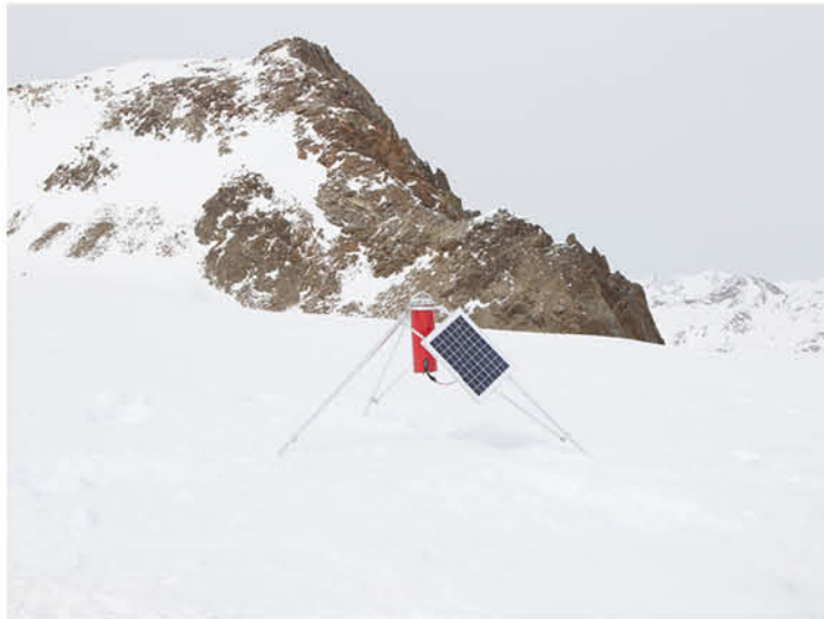
The measuring units installed on the glacier are solar-powered devices based on an Arduino micro-controller. They have been designed to record precise changes in altitude as well as a range of other environmental data, useful to understand the weather conditions on the glacier.
